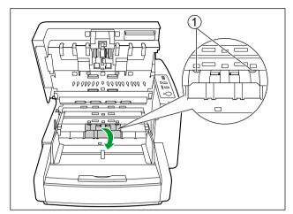
**4.** Remove the double feed prevention roller (1) in the direction of the arrow.
